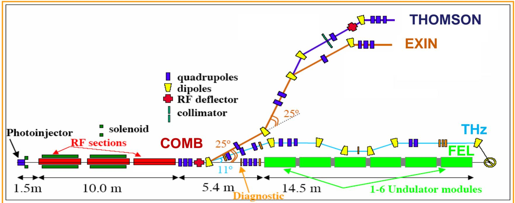
**Test Facility** composed by a **high brightness** electron linear accelerator and a high power laser (FLAME)
