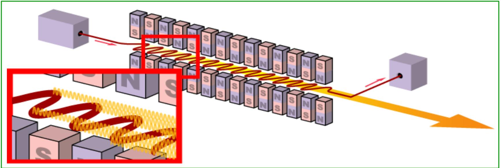
Tunable laser with frequency ranging from microwaves to X-rays
